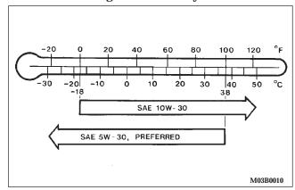
Use engine oil with proper thickness for the outdoor temperature where you will be driving.
